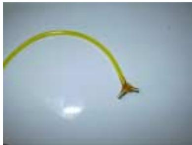
28. Connect the two yellow lines on the retracts to the y-connector from Step 27 attached. Stick the excess tubing inside the fuselage to get it out of the way for now.
