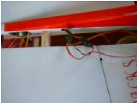
133. Tuck the excess cable back into the wing, not the fuselage. If you need to, it will e very easy to remove the wings for transport.
