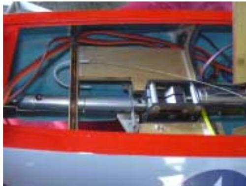
149. Run the charge leads from your switches through the hole in the rear nose gear former up into the nose gear area so you can get to them for charging.
