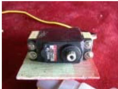
76. Put a horn into place to establish where the horn will emerge from the servo cover door.
