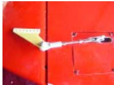
90. Put a piece of masking tape on the surface of the rudder where the horn will go. This tape will protect the surface while you work there, and keep any markings you need to make from being on the surface itself.
