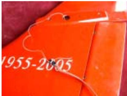
97. Fair the extension into the string with masking tape as shown to keep the connector from snagging on the internal structure.
