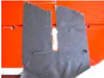
118. Add a bead of glue to each side of the control horn. Be sure to use your nozzle to inject glue into the small holes in the horn, they need to be filled with glue for proper strength of the joint.
