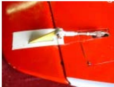
94. You will need to feed a heavy-duty 22-gauge 36-inch extension through the right side boom for the elevator servo. Feeding extensions through the structure can either be a very tedious, time-consuming, and frustrating process, or you can follow my technique and it will only take a minute. All you need is a weight such as a wheel collar, a little bit of string such as dental floss, and a little bit of masking tape. Tie the wheel collar to the string, and read on.
