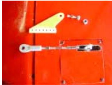
89. Bolt a horn into place, and adjust the linkage to the correct length.
