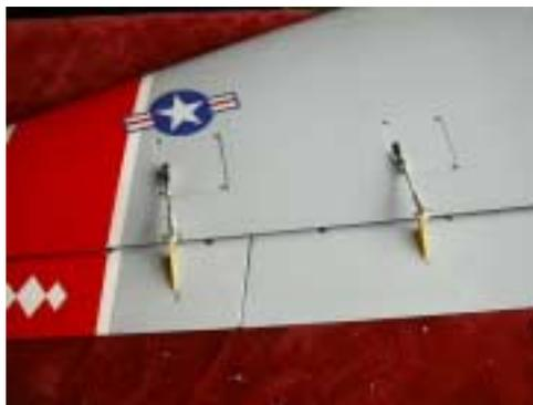
109. Install the flap servo into the right wing normally. For the left wing, do this: Cut two scrap plywood blocks as shown, the same width as the existing servo mounts, but about 1" long.
