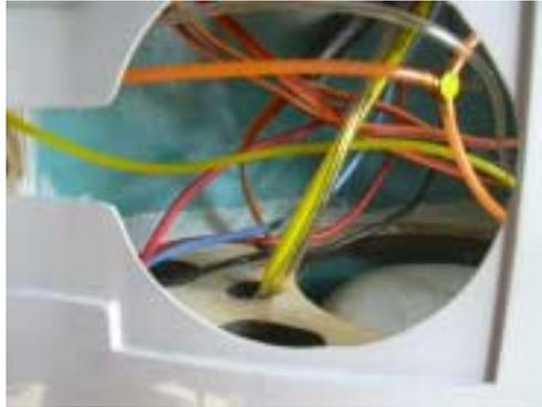
191. Use tie wraps to neaten up and secure all wiring and tubing in the wheel wells. Nothing should be flopping around. Be careful not to squeeze any of the pneumatic lines. Separate and layer the servo leads, pneumatic lines, turbine electronic lines, and fuel lines, for neatness and easier service, and to keep any potential electronic interference at a minimum.
