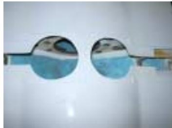
22. Carefully align the retract assemblies, double check that they clear the wells properly, and mark the four mounting holes for each retract.
