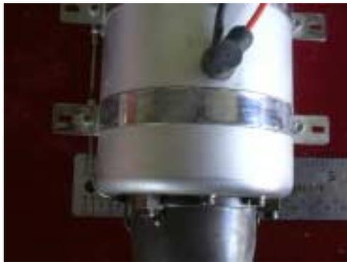
159. Subtract the measurement of your engine from step 158 from the width of the plate. Divide this by two. Measure that dimension in from each side of the plate and make a line there. In this case, we measured 4" between the holes in the turbine bracket, subtracted it from 6 5/8", leaving 2 5/8", and divided 2 5/8" by two to get 1 13/16", and made a line at 1 13/16" in from each side.
