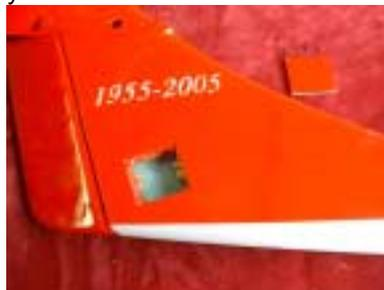
68. Test fit your rudder servos. You want a metal-gear, high powered mini servo. A standard servo will not fit, and full micro servos generally lack
