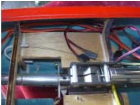
150. Check all your wiring and plumbing beneath the radio tray, then secure the tray with the provided two screws. Note how the airlines go around the side of the tray and over to the bottom. Be extra careful about pinching or kinking airlines.
