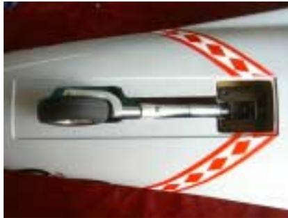
38. Mark and drill pilot holes in the nose gear mount for the nose gear assembly.
