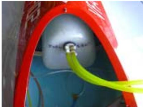
140. Adjust the size of the hole in the radio tray to fit your UAT or header tank. A sharp Exacto with a new blade will cut the plywood very accurately with a few strokes.
