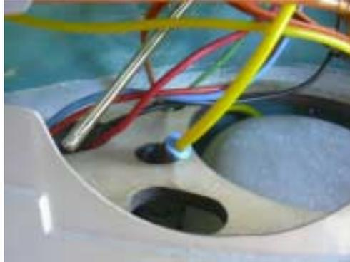
190. Connect the fuel line for the engine to the fuel solenoid, going through the hole in the bulkhead as shown.
