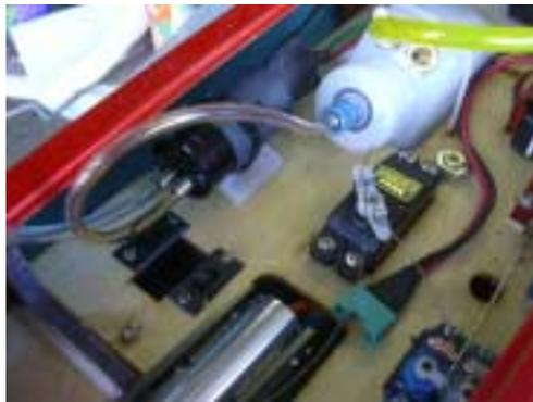
182. Run the output side of the fuel pump to your manual shutoff valve and then to the fuel solenoid.
