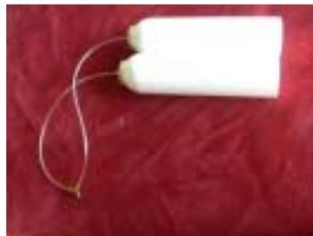
55. Install the air tanks into the fuselage on either side of where the main fuel tank goes. Do not block the holes in the rear former. Silicone is a good way to install these tanks, in case you need to remove them later for servicing. You may also use epoxy.
