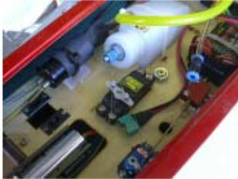
181. Connect the input side of the fuel pump to the UAT
