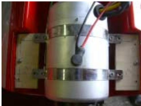
166. Remove the plates. Put a fuelproof finish on them in case of fuel spills.
