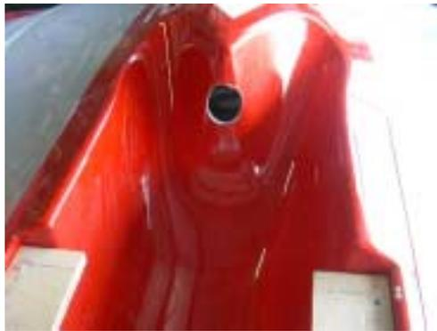
164. Take a scrap piece of airline tubing about four inches long. Cut a notch out of it with a sharp razor, and fit it around the edges of the hole you made, and CA it into place. This will serve as a grommet to keep the sharp edges of the fiberglass hole from cutting your wiring and tubing.
