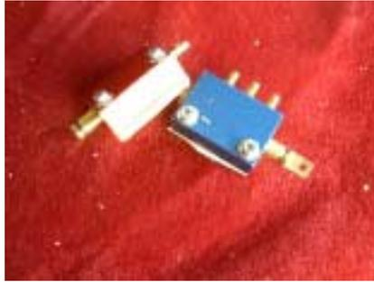
49. Glue the blocks with the valves into place using thick CA. Notice how the valves are staggered to keep from hitting each other, and to keep the airlines that will be attached from interfering with each other.
