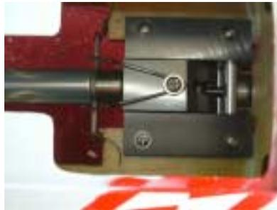
42. Flip the plane over. Remove the radio tray. Put the screws back into place in the fuselage to keep them from getting lost.
