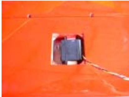
101. Fit the supplied aluminum mounts to the servo, using the supplied screws. Do not over tighten and strip the screws. Do not use any grommets or other servo hardware. Secure the screws with Loctite.
