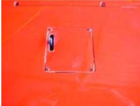
107. Fit the linkage, control horn, and slot for the control horn as you did for the rudders. Again, you can wait till later to glue the horns.
