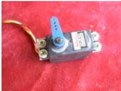
104. Fit the servo into place, with the servo lead coming out the right side (from the top) of the stabilizer assembly.
