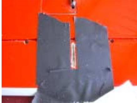
117. Fill the slot completely with Hysol. Inject the glue as far in as you can go, it's much better to have excess glue here than too little. This application is another great reason to use the Hysol glue gun and nozzles, it is very difficult to get the glue down inside the slot without a glue gun.
