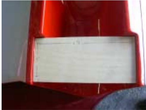
157. Drill pilot holes and install the plate with three screws on each side. Be careful when you drill not to go through to the bottom of the fuselage.
