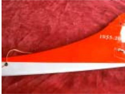
99. Remove the elevator servo cover.
