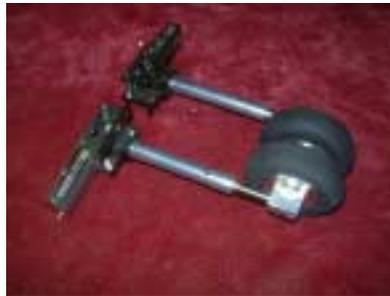
19. Use your hand pump to pressurize the gear very slightly until it is not locked either up or down, but can move freely in the middle. Insert the landing gear into the mounts and wells and check the fit.
