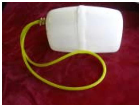
138. Test fit the fuel tank and adjust the velcro strap installed at the factory. Keep trying until the strap is a nice tight fit when you slide the tank in.
