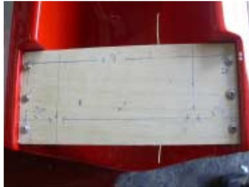
160. Remove the plywood plate. Cut on the lines you made and re-mount the plates with one screw on each side.
