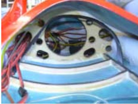
139. Slide the tank into place. Make sure it is square and butted against the former behind it. Use some silicone glue for extra security. Silicone keeps the tank in place, but still leaves it easy to remove in case service is needed.
