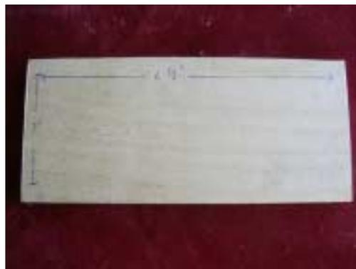
156. Test fit the plate between the engine bearers at the rear of the fuselage.
